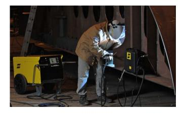
The welding properties of these units are configured to meet the requirements of welding with celluloid electrodes. The arc is very flexible when starting from the lowest currents.
